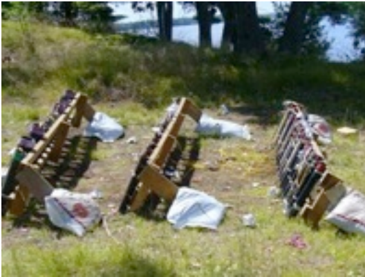
Cannons aimed and sand bagged in the photo below. Note the yellow wire that connects the mortars to the control panel.
